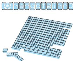
**2** Insert the characters into the character holder one at a time from the right end, making sure they are facing the correct direction.
