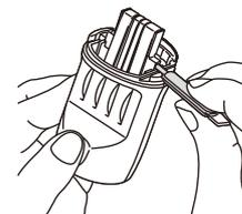
Remove the holder and insert nozzle into hole and gently squeeze all the ink into stamp.
